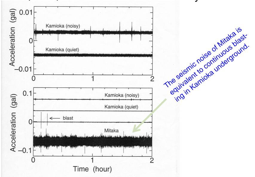
When the 2 0 m interferometer was moved from Mitaka to Kamioka mine, the noise at 100Hz was decreased by 4 orders and the spectrum limit by the anti-vibration system was achieved at frequencies less than 100Hz.
