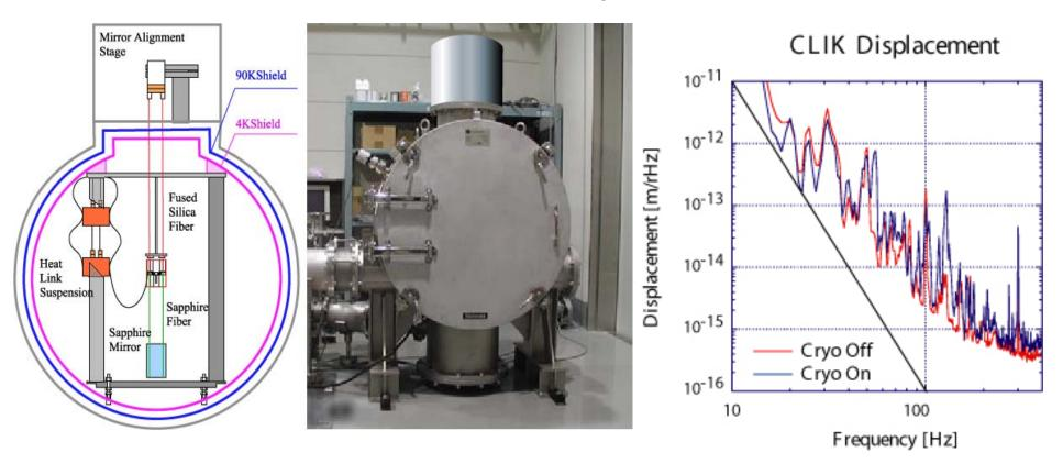
This result makes us to develop quieter refrigerator and softer heat link design.
