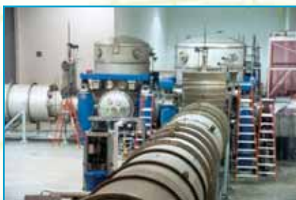
A view of the interferometer's interior. This shot shows the vertex of the L.
