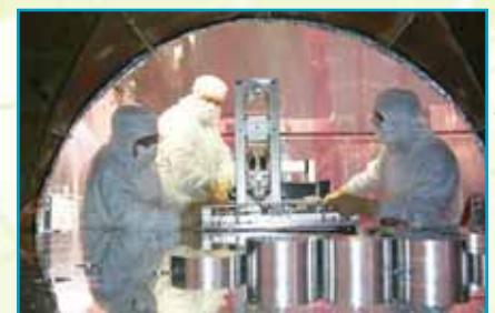
LIGO staff install a mode-matching mirror and suspension into a vacuum chamber.
