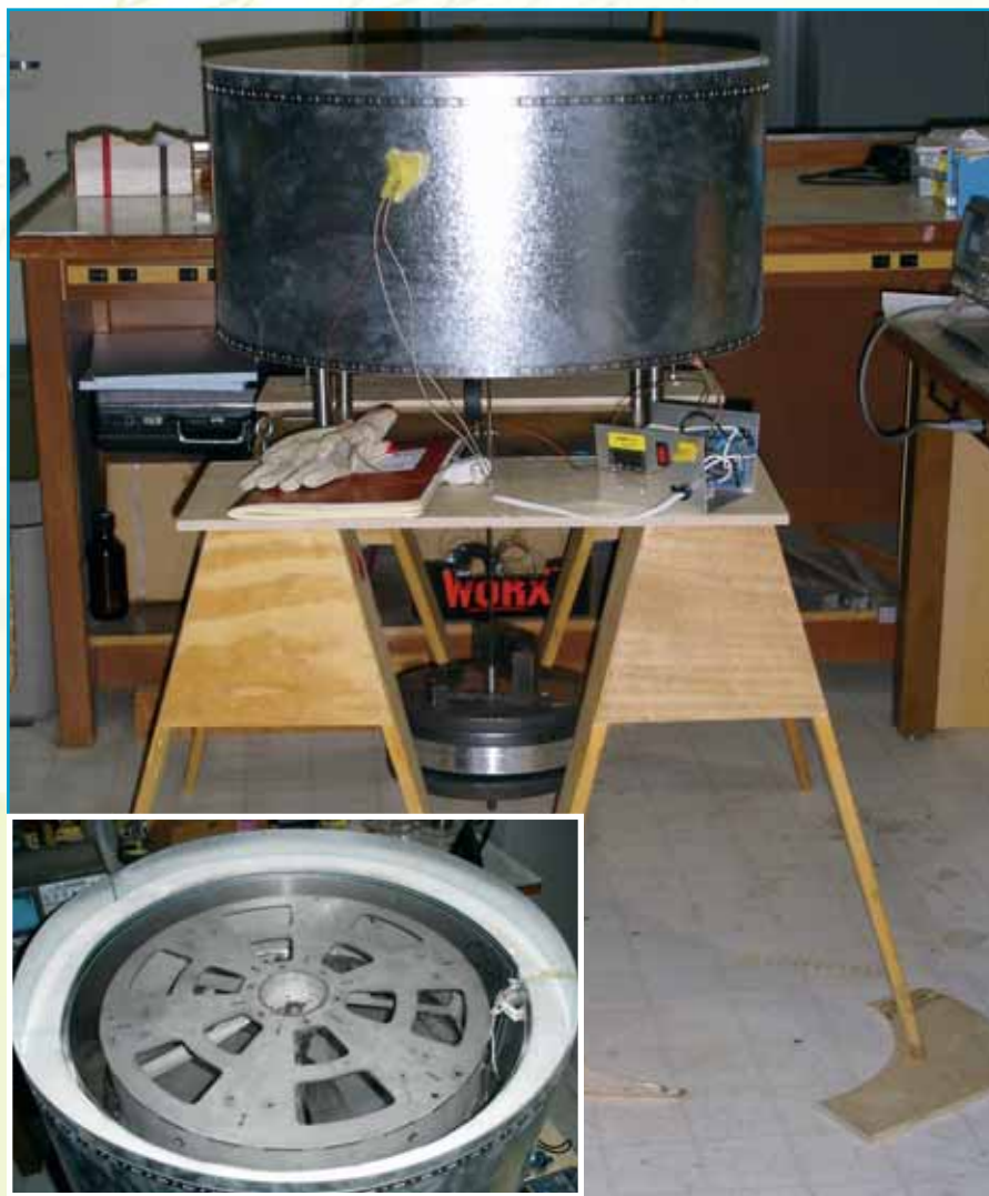
The oven that Nicky built to test the creep property of a metal alloy. The temperature controller sits on the table; the payload hangs below. Inset: A view of the oven's interior.
