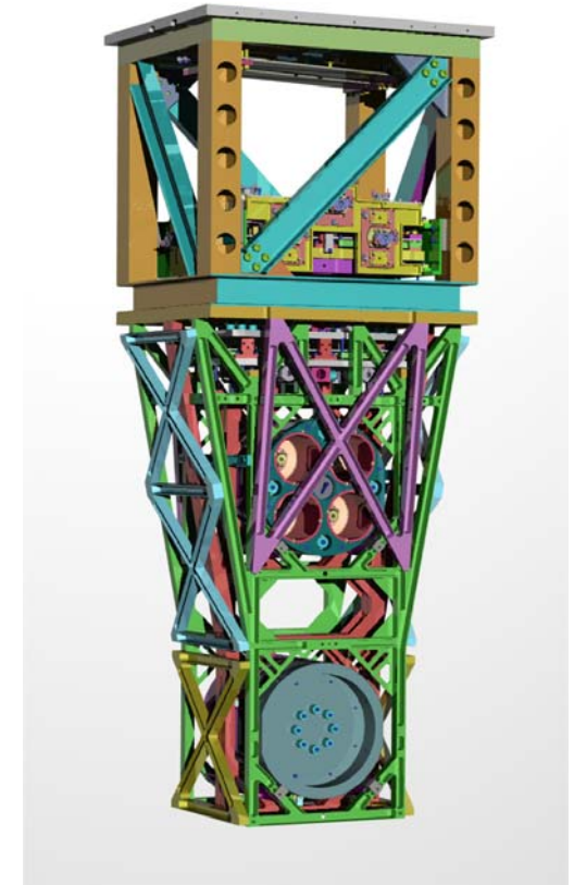
Quad noise prototype (all-metal mass version) within support structure
