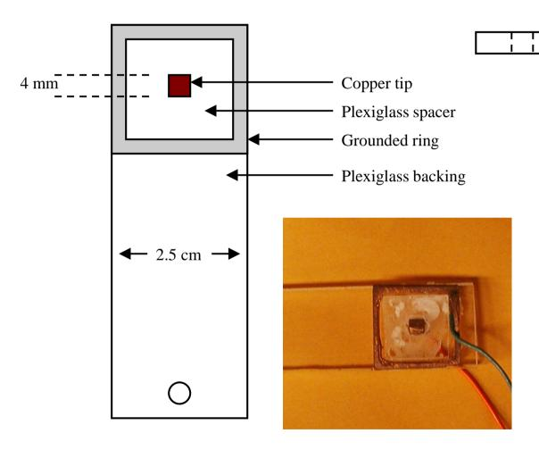
Grounding ring too large, coil on chopper prevented the probe from getting closer than 1 cm.
