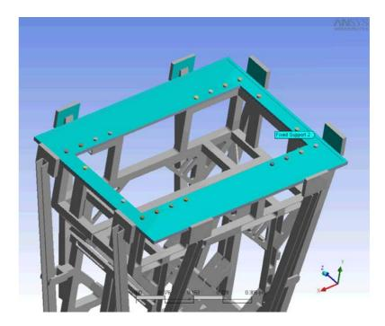
case two. Fixed supports are maintained on the outriggers assembly pads to the implementation ring (implementation ring not included in the model) and on the entire surface of the top plate.
