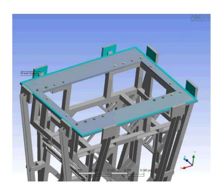
case one. Fixed supports are maintained on the outriggers assembly pads to the implementation ring (implementation ring not included in model) and around the perimeter of the top plate.
