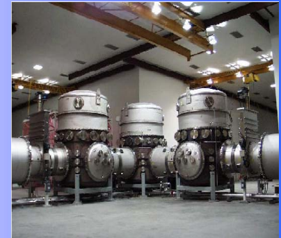
Whole Interferometer Enclosed in Vacuum
