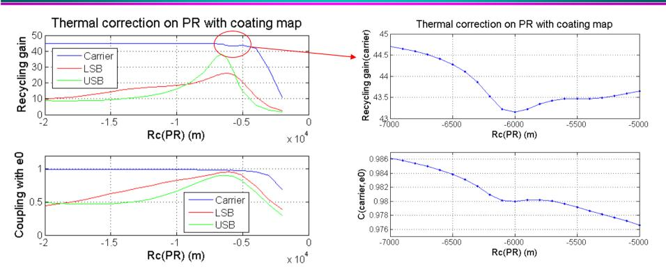
Why does the carrier coupling with a perfect TEM00 of waist 2cm decrease when the recycling mirror curvature radius is around -6km?
