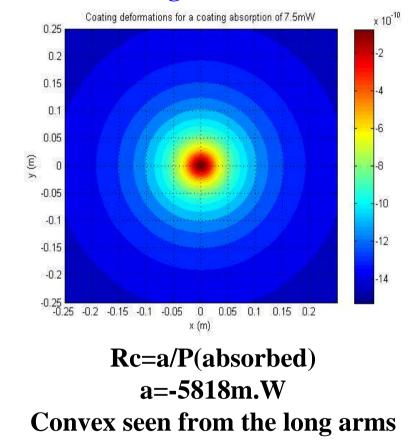
The thermal lens produces an effect 16 times larger than the coating deformations.
