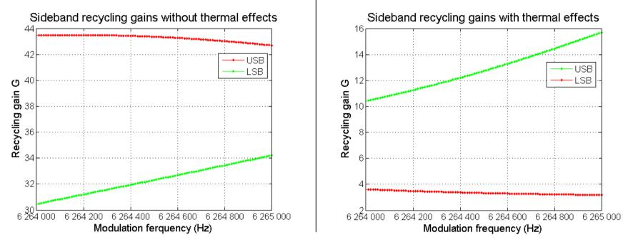
**Conclusion :** A weak modification of the modulation frequency cannot correct the shift between the recycling gains of the sidebands before and after the thermalization.
