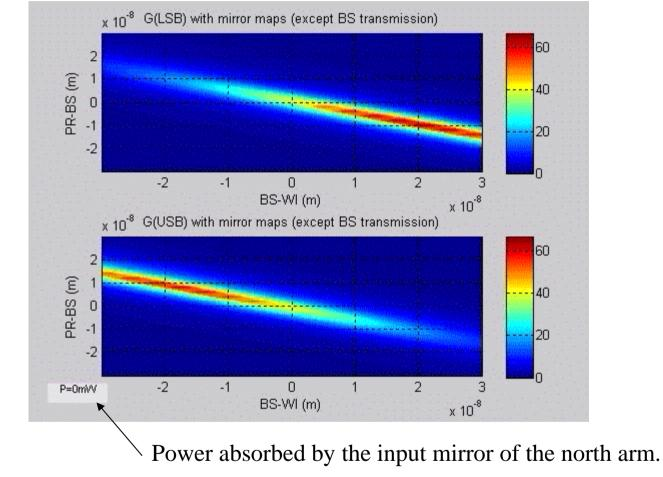
**Method to calculate the error signals:**  $V = dx^2 \times \sum (Carrier \times LSB^* - Carrier^* \times USB)$ Sp = Im(V) Sq = Re(V)
