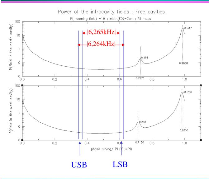
When the modulation frequency increases from 6,264 to 6,265MHz, the storage coefficient of the sidebands should decrease.
