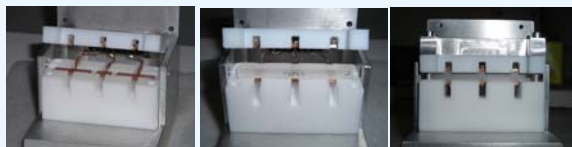
eLIGO: 3 frequencies / 1 crystal / 3 separate electrodes
