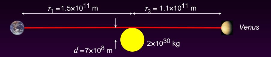
Light or radio beam passing by limb of Sun is delayed by
