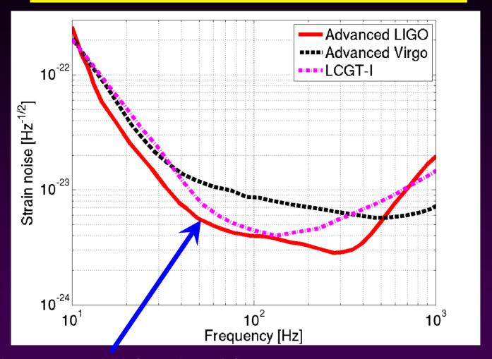
Choose 50 Hz for signal frequency Integrate for a long time  $\Rightarrow$  SNR grows as  $\sqrt{T}$
