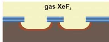
3 - dry undercut of Si substrate
