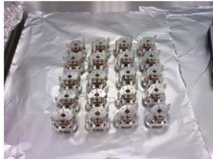
Assembled BOSEMS at testing station
