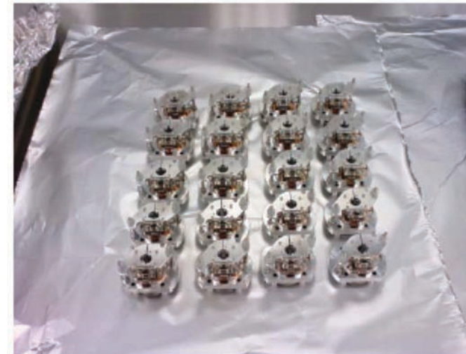
Assembled BOSEMS at testing station
