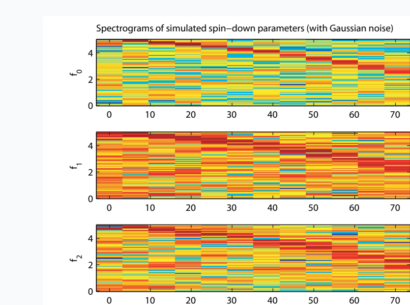
Figure 6: Spectrograms of the spin-down parameters of a synthetic signal with Gaussian noise added, resulting from the time series in Figure 5.
