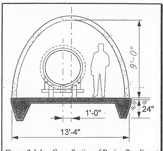
Figure 2.1-1 -- Cross Section of Design Baseline at Hanford
