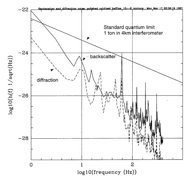
Baffle backscatter BRDF =  $4.8 \times 10^{-3} \text{ sr}^{-1}$  Polished oxidized baffles
