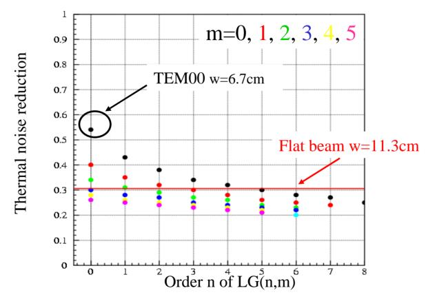
Thermal noise reduced by a factor 3 to 5 with respect to present Virgo configuration
