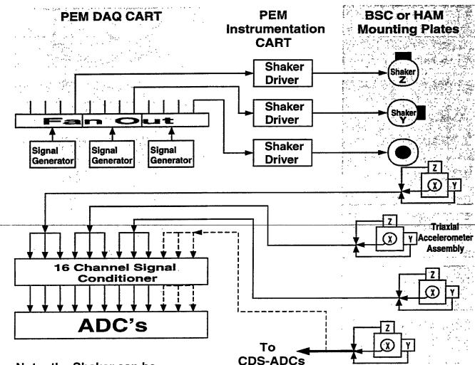
Note: the Shaker can be PZT or Electromagnetic Shaker
