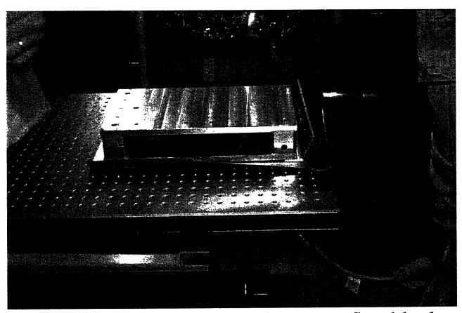
HAM - LOS height adapter sitting on Teflon blocks and Teflon highway on the straddle lift. This is set up to transfer the LOS structure from the transport cart.
