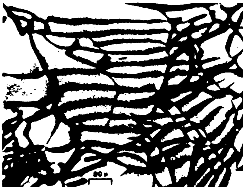
Fig. 7. X-ray topograph of edge dislocations gliding under the stress in a sapphire single crystal. Ag K_{\alpha 1} radiation.
