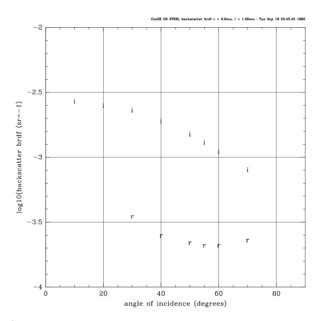
Figure 1 Glaze on steel backscatter brdf at 0.63 (r) and 1 (i) micron wavelength.
