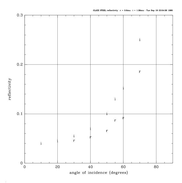
Figure 2 S polarization reflectivity of the glaze on steel. The p polarization reflectivity vanishes near the Brewster angle so between 40 to 60 degrees incidence the average reflectivity is close to 1/2 that plotted.
