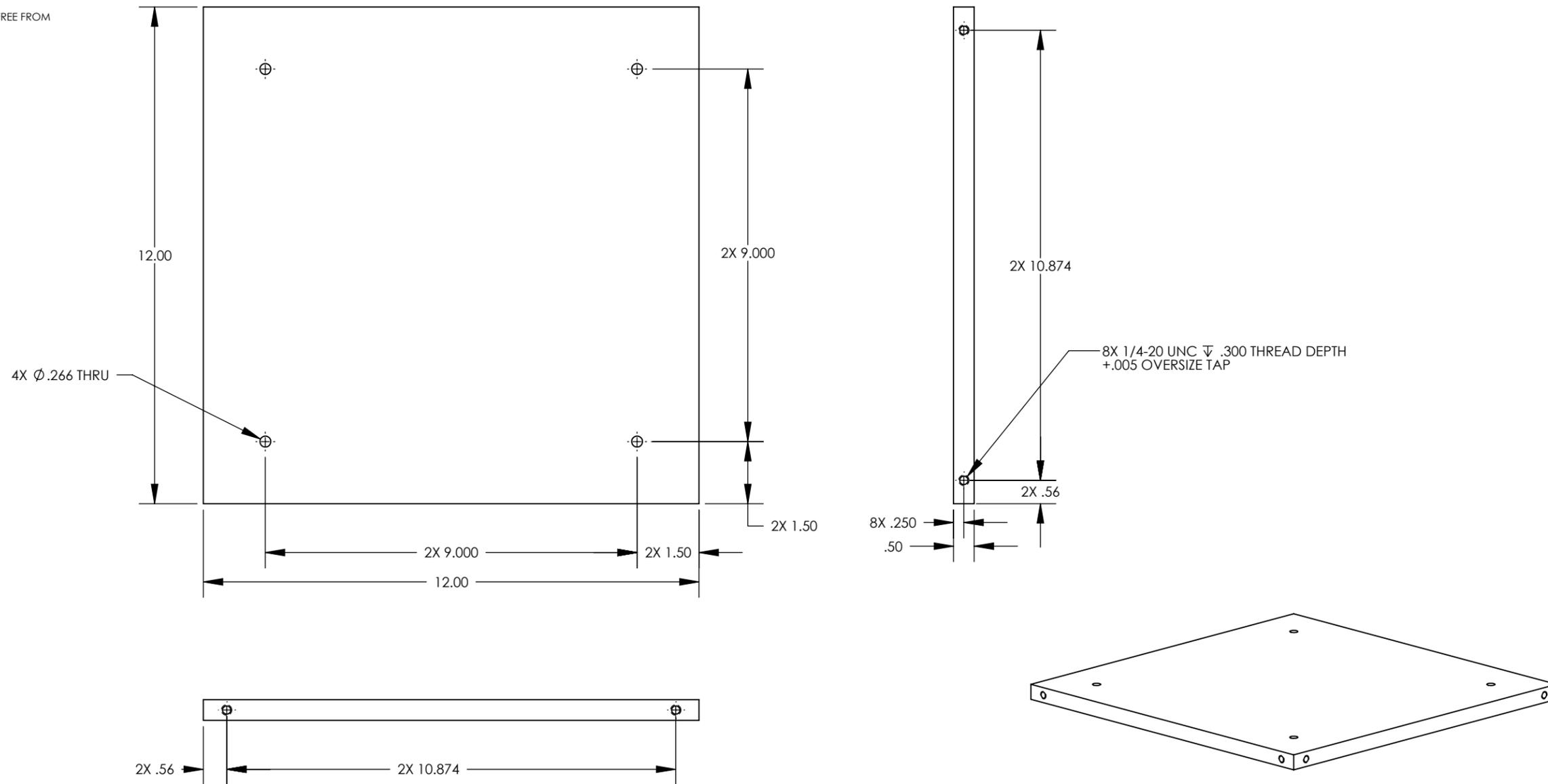
D1100772 Top, Shack-Hartman Pedestal, PART PDM REV: X-002, DRAWING PDM REV: X-001
