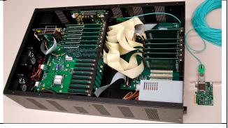
Figure 1: aLIGO IOC and PCIe Fiber Link
