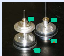
Figure 4. The aluminum "fuse-ends" glued to 2mm silica stocks (1) were fastened to the end cups (2).
