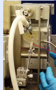
Figure 8 (on the right): GEO prototype suspension with metal masses (5.6 kg). The ear holder is bolted in place and is set up for flame welding of silica fibres. The ears are glued to an aluminium holder by an epoxy Araldite 2012 or by heat-proof adhesive Resbond 989F.
