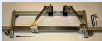
Figure 6: Fibre cutter / holder having three x-y-z stages for accurate adjustment while welding
