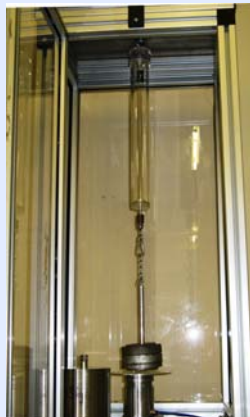
Figure 5. The fiber is tested (in situ) to prove its durability; the bottom "fuse-end" is not fastened to the polycarbonate tube; the container is used as a protective shield here.
