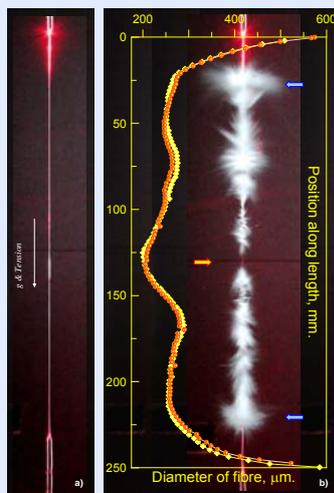
Figure 3. Two photos of a fibre before (a) and during (b) breaking. The diameter profile vs position along the length superimposed with breaking photo b. The initial breaking point shown by a yellow arrow.
