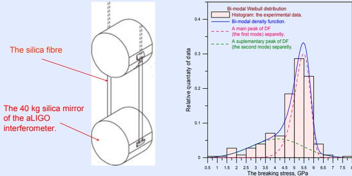
Figure 1. The lower (fully monolithic) stage of aLIGO test mass suspension.
