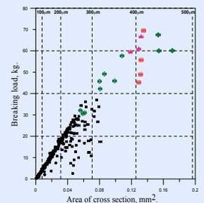
Figure 8. The data shown in fig. 7 presented as breaking load vs cross sectional area. The vertical grid shows here the fibre diameter. Laser pulled fibres heated for alignment manifest a large spread of data.
