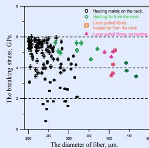
Figure 7: The breaking stress of fibres heated for alignment a few mm outside of their neck or not heated at all. Fibres pulled using the H<sub>2</sub>-O<sub>2</sub> flame and CO<sub>2</sub> laser are presented on this graph.
