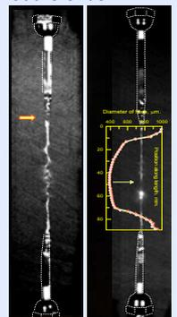
Figure 9. The breaking of two similar fibres that were pulled sequentially on the CO<sub>2</sub> laser machine. The low contrast details are contoured by dotted lines. a) – the stocks were heated by flame a few mm away of the necks; b) – no heating (no alignment) was employed.
