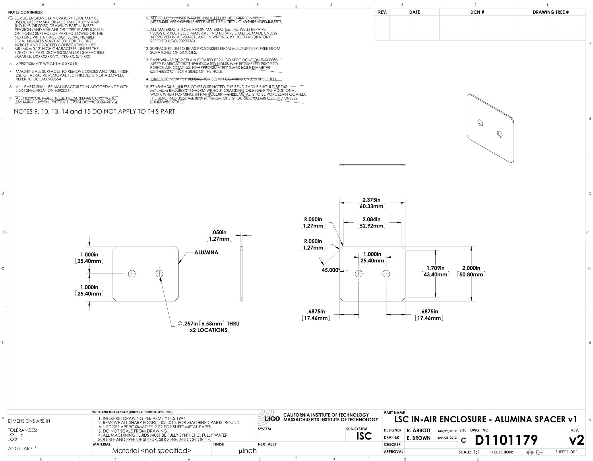
8 D1101179\_LSC\_AIR\_v2 Enclosure - alumina spacer, PART PDM REV: , DRAWING PDM REV:
