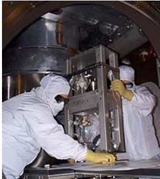
FIGURE 1. Mirror Installation Begins on Four-Kilometer Interferometer at Hanford.
