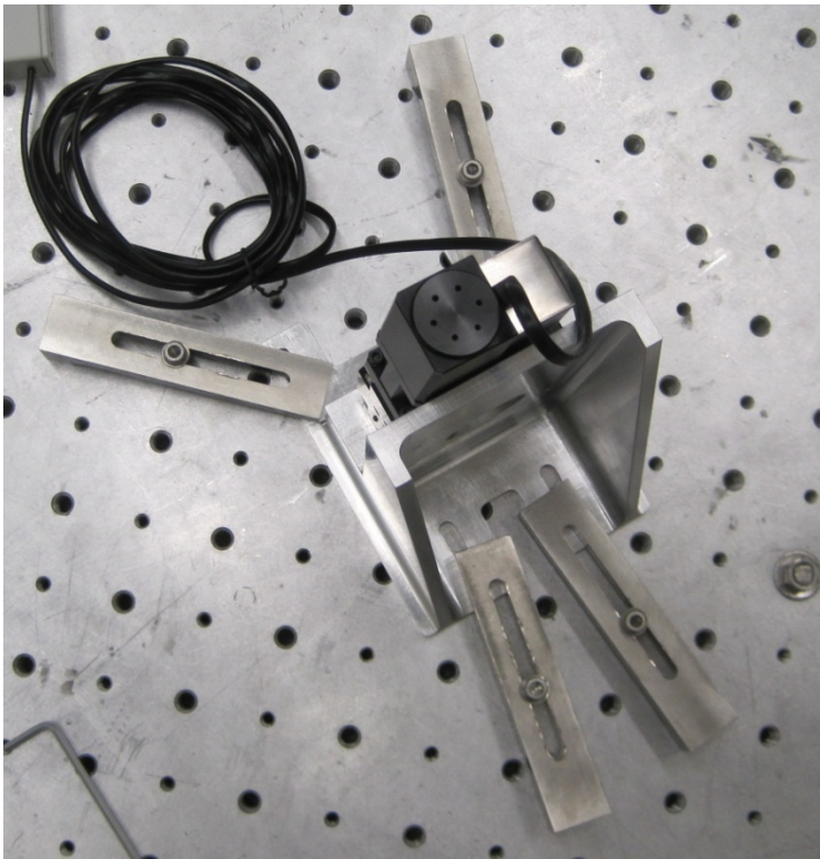
Figure 1.1: This is the clamping arrangement used for this test.
