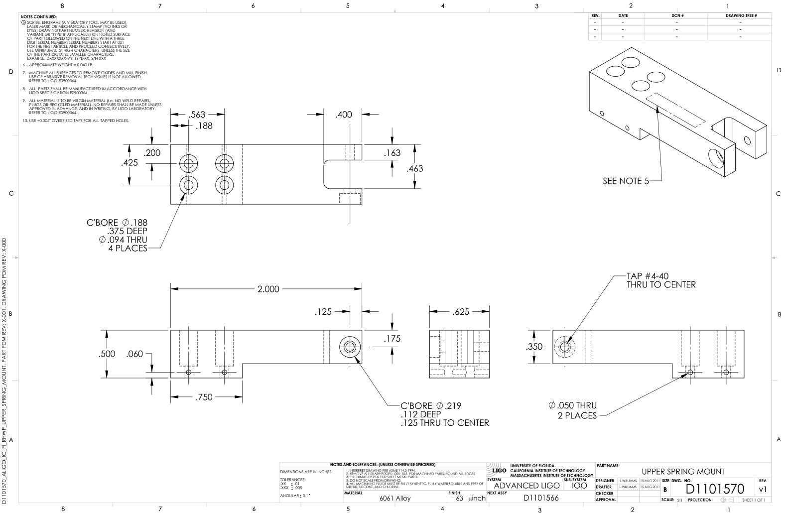
DRAWING PDM REV: PDM REV: X-001, **B** PART MOUNT, ALIGO\_IO\_FI\_RHWP\_UPPER\_SPRING\_ D1101570\_
