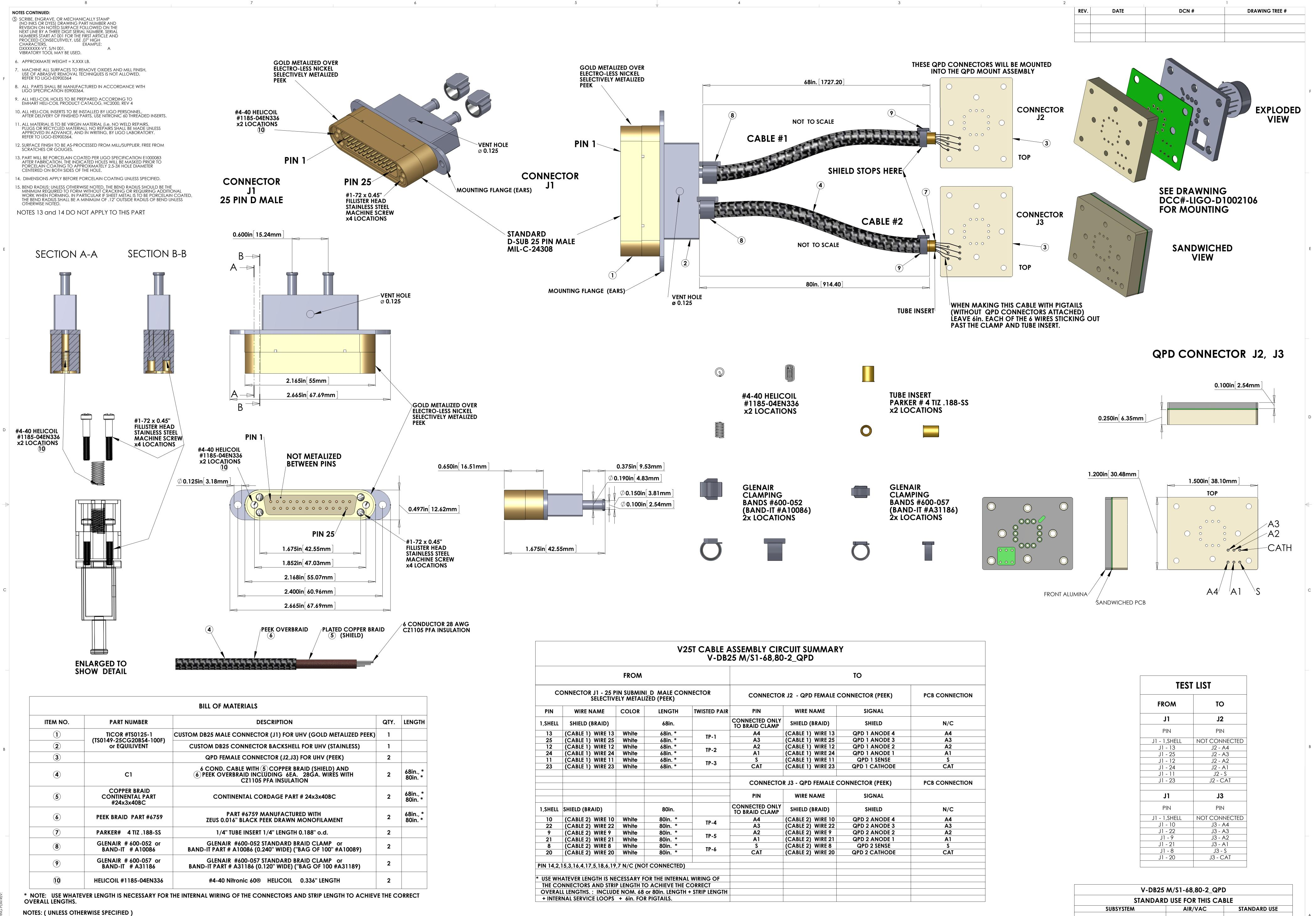
A. MATERIAL: a. J1 CONNECTOR SHELL - GOLD OVER ELECTRO-LESS NICKEL SELECTIVELY METALIZED PEEK VICTREX 450GL30. **b. BACKSHELL - STAINLESS STEEL WITH VENT HOLE.** c. CONTACTS - BERYLLIUM COPPER ALLOY C17300
