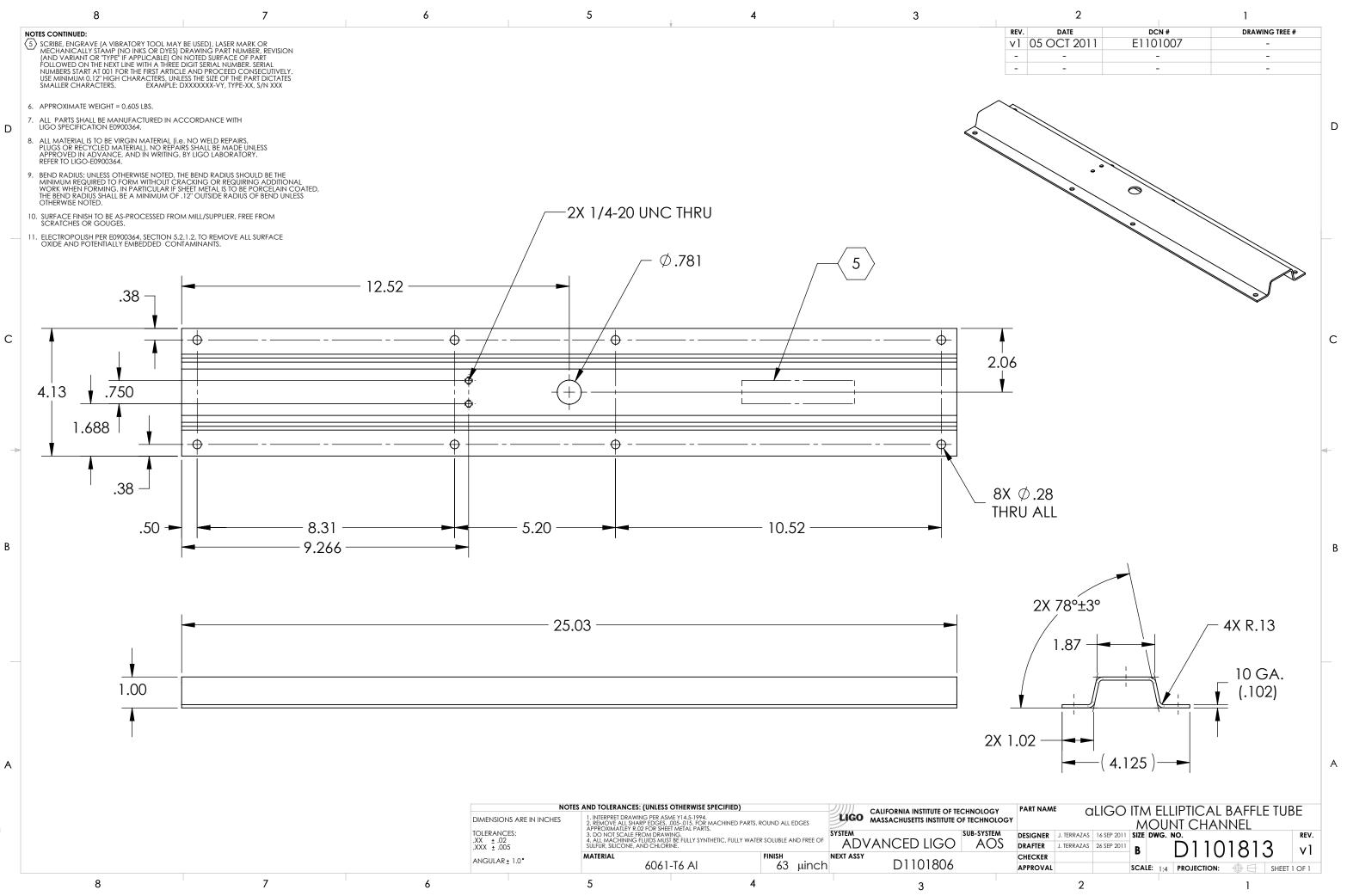
PART PDM REV: X-030, DRAWING PDM REV: X-017 8 CHANNEL, aligo itm elliptical baffle tube mount **>** D1101813
