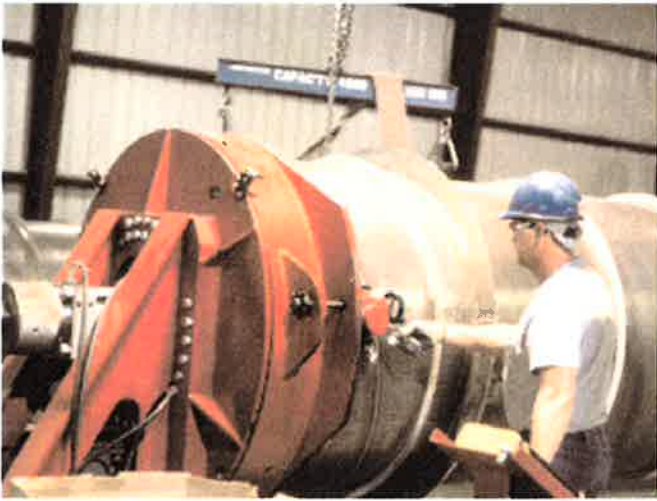
Figure 3 - Machining Tube Ends
