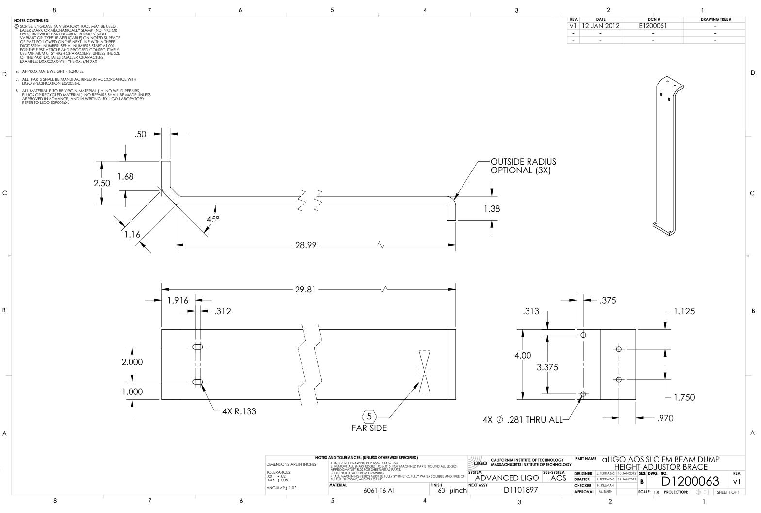
DRAWING PDM REV: X-002 PART PDM REV: X-002, **B** ADJUSTOR BRACE, FM BEAM DUMP HEIGHT \_aligo Aos slc F D1200063
