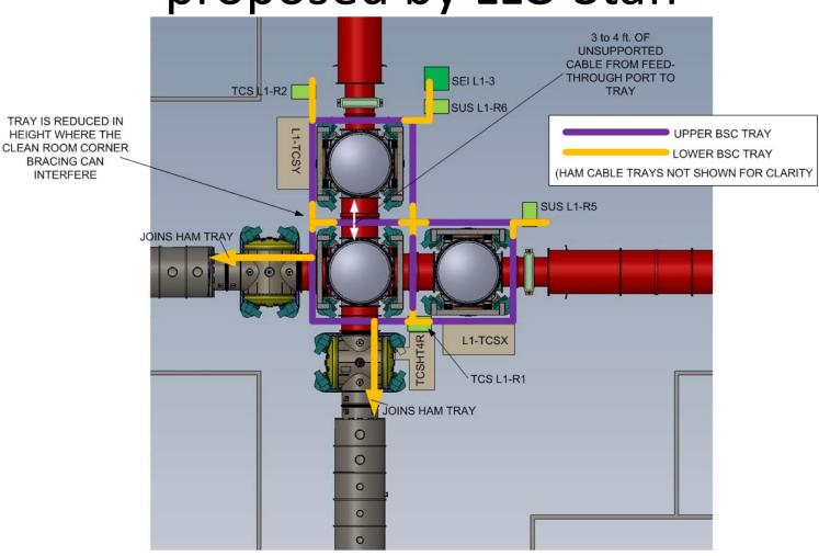
From the LLO Corner Station Layout, D0901466-v4, and (in leau of L1 LVEA Rack & Cable Tray Layout, D1003141) the H1 H2 LVEA Rack & Cable Tray Layout, D1100024-v2 G1200110-v3
