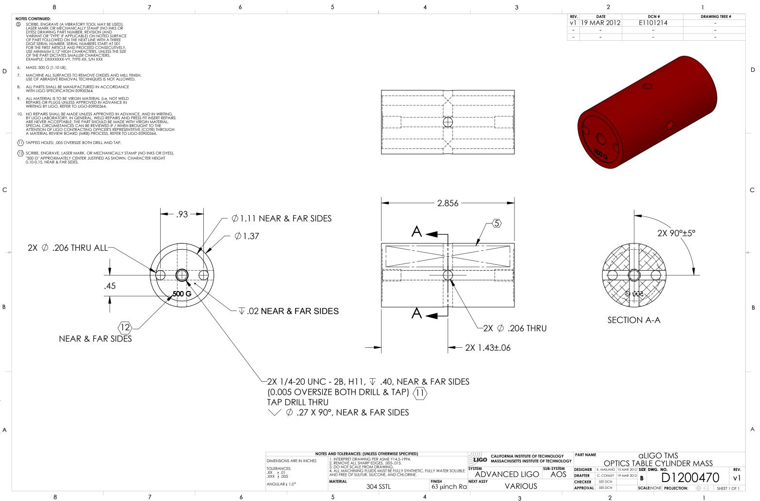
D1200470 aLIGO TMS Optics Table Cylinder Mass, PART PDM REV: X-000, DRAWING PDM REV: X-002 A
