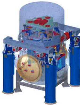
Figure 1 LBSC3 chamber with vacuum equipment and HEPI
