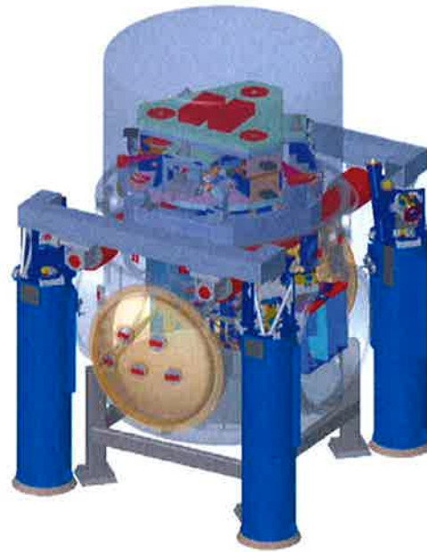
Figure 7 LBSC1 top-level assembly with transparent chamber for clarity. Refer D0900492: aLIGO Systems, BSC3-L1 Top Level Chamber Assembly
