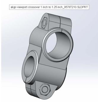
16 of these they connect the horizontal tubes to the foot post 4 per assembly and there are 4 assemblies
