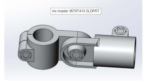
12 of these for the horizontal tube 1 1/4 inch to the down tube 1 inch dia these are bored out and start life as one inch
