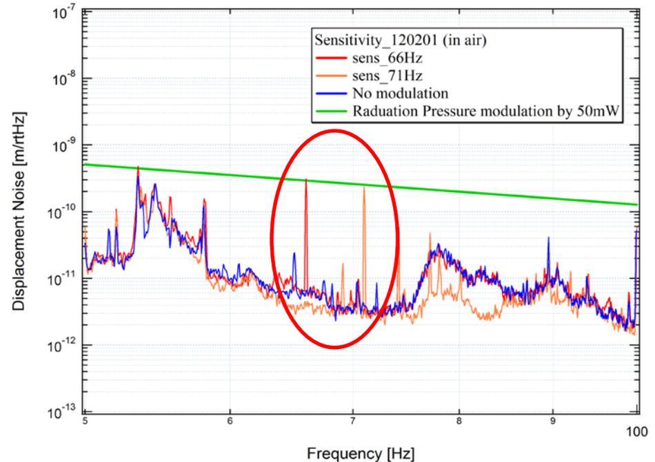
Large amplitude of displacement comparing with floor noise is observed
