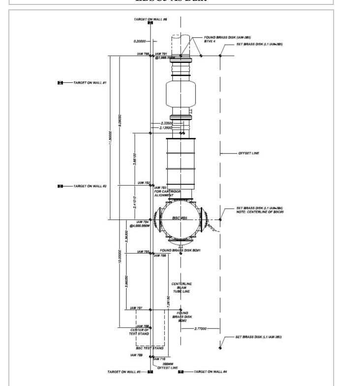
Figure 2: Monument Layout for Y-End Station, inc. Test Stand (from E1100374)
