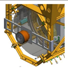
Figure 4: Retro-reflector Assembly attached to Quad Suspension Structure
