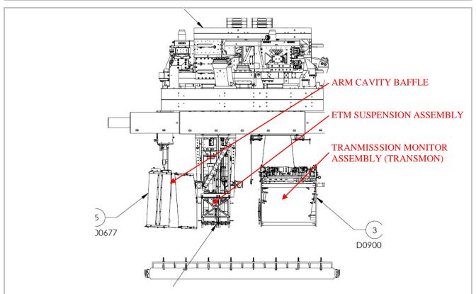
Figure 3: The LBSC5 cartridge assembly (from D0900506)
