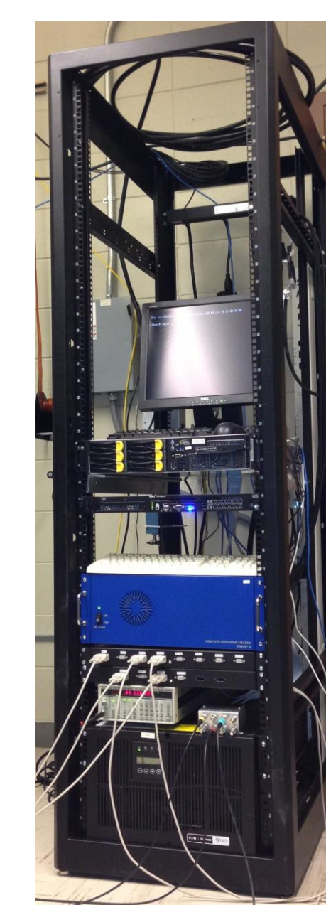
Fig 9: Syracuse University Digital control rack: from top to bottom it contains a front end computer, a boot server, the PXI-x expansion chassis, the in-house analog filter box, a GPS-locked clock and a UPS.
