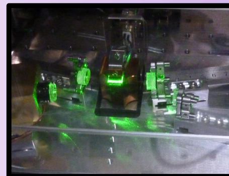
The Optical Parametric Oscillator of the LIGO squeezer (ANU design)
