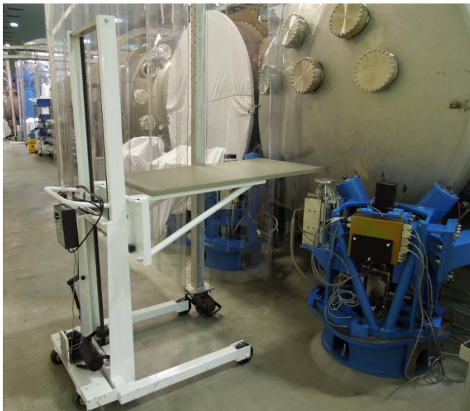
Figure 1. White lift table at LLO positioned in front of HAM6
