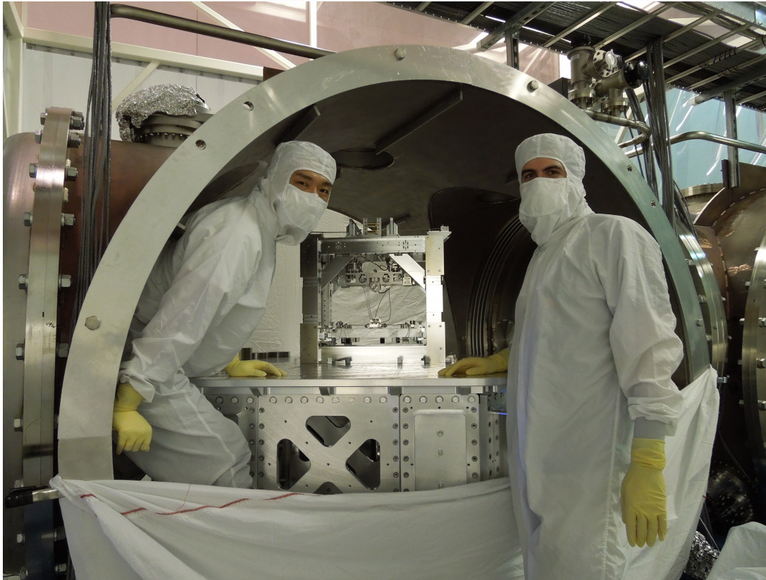
Output mode cleaner installation (more pictures from Zach)
