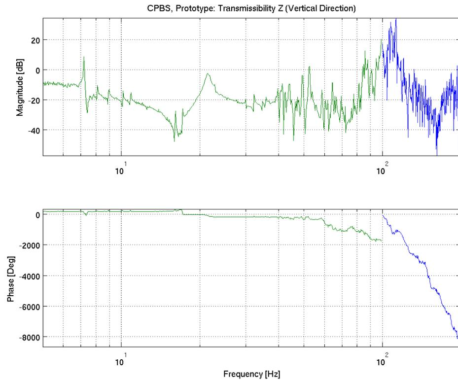
Transmissibility along the vertical direction somehow orthogonal to the laser beam axis
