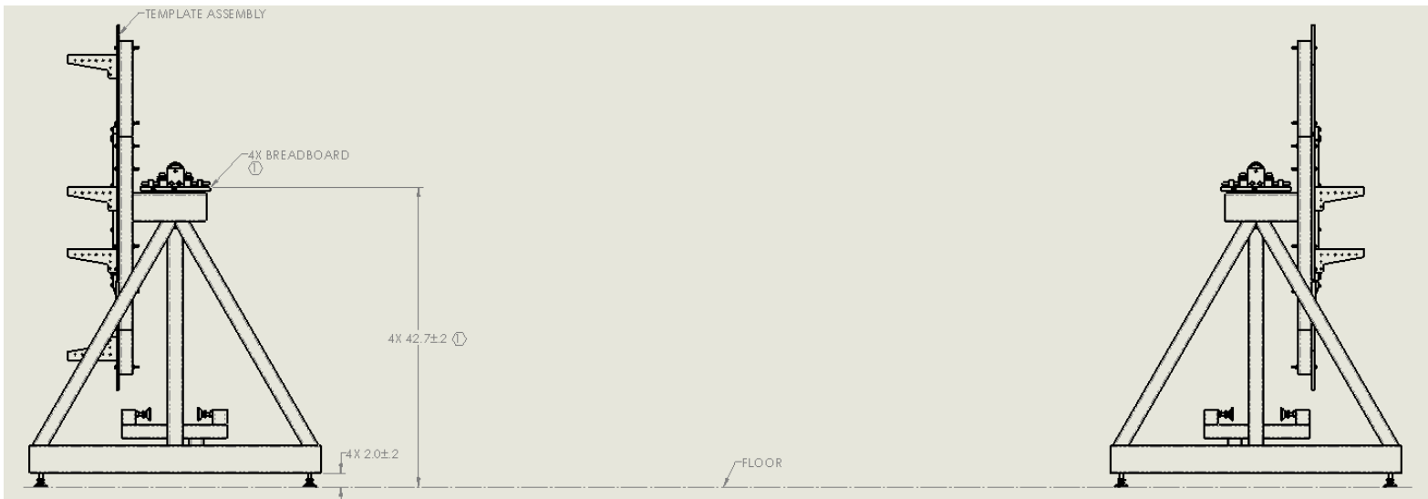
Figure 3 Pre-Alignment Setup, elevation view, showing the two Periscope Support Assemblies (Cradles).
