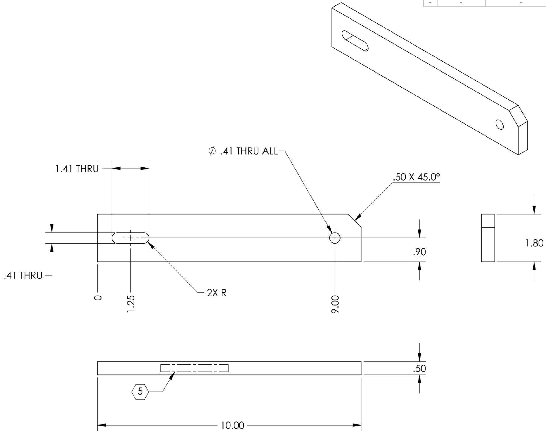
D1300676 Tie, Riser, Storage, HAM1, 3rd IFO, aLIGO, PART PDM REV.: , DRAWING PDM REV.:
