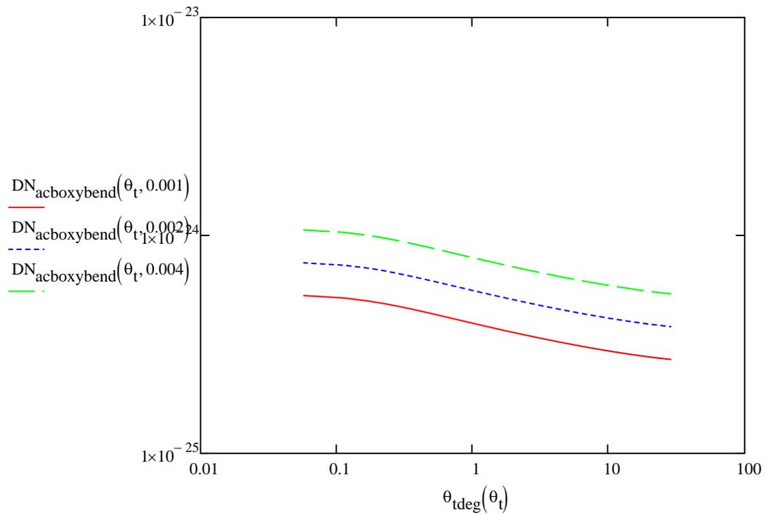
**Power Scattered from the louver portion of baffle**
