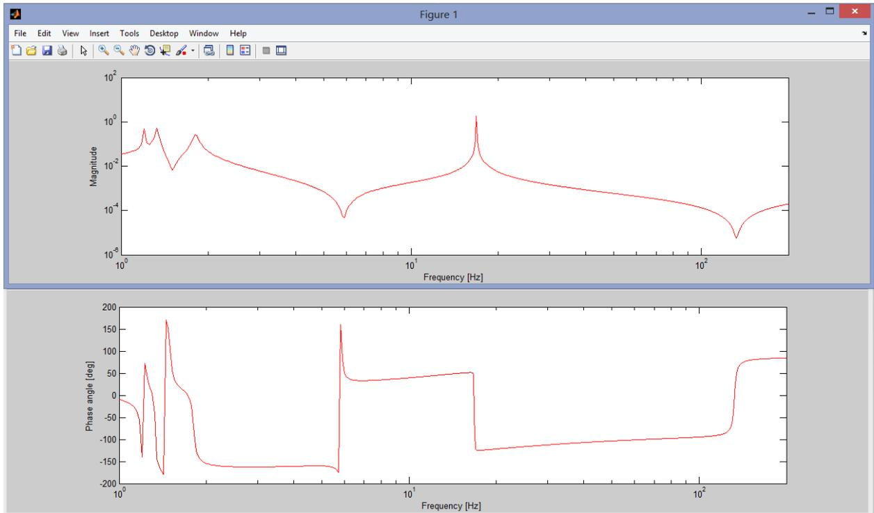
Figure 3: Filter Definition in Matlab
