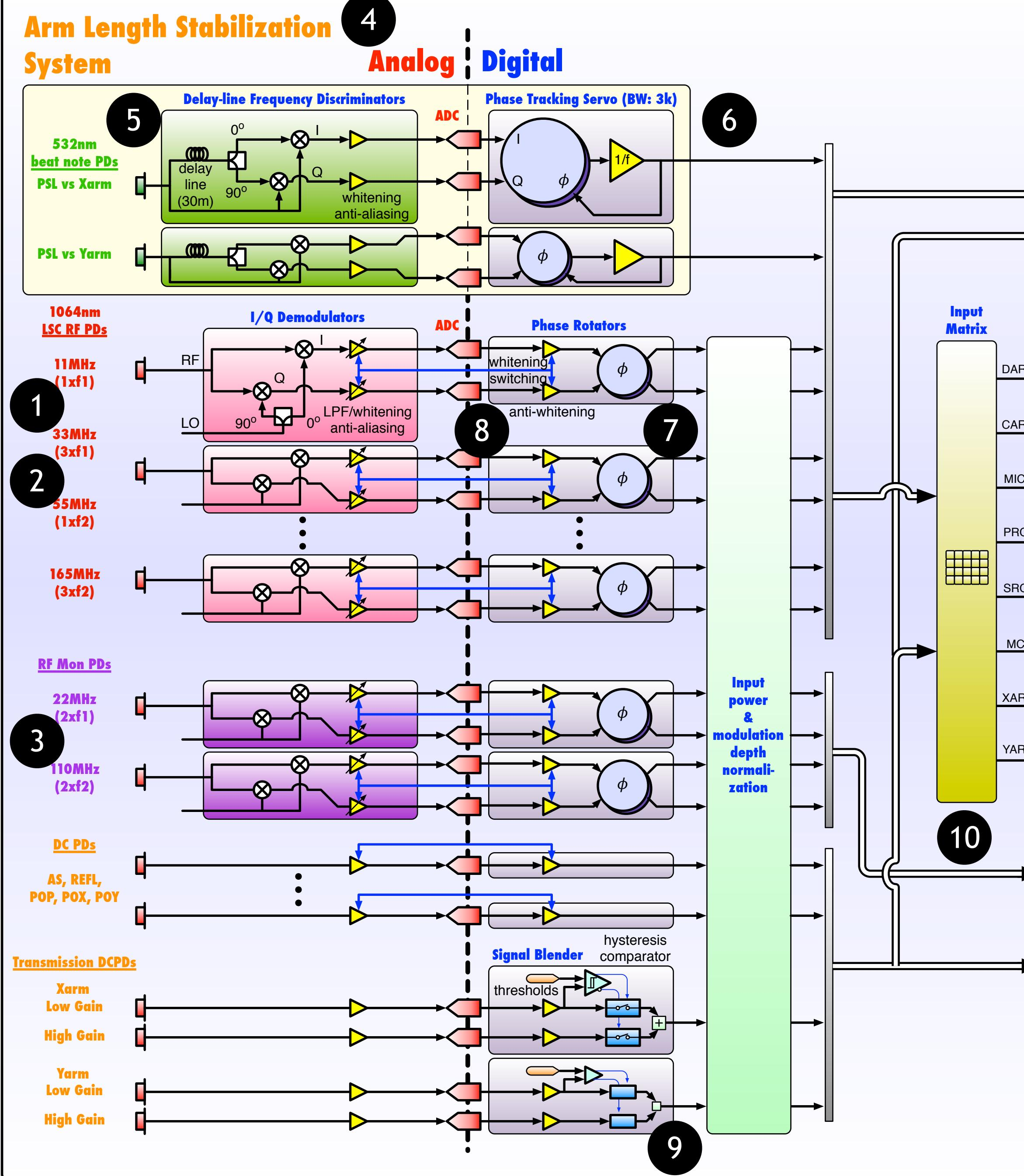
**11 Normalization matrix:** Intracavity power monitoring signals are selected for use in normalizing length error signals. This normalization increases the linear range of the error signals during lock acquisition.
