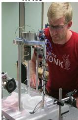
We measure properties of the mirrors to minimize thermal noise
