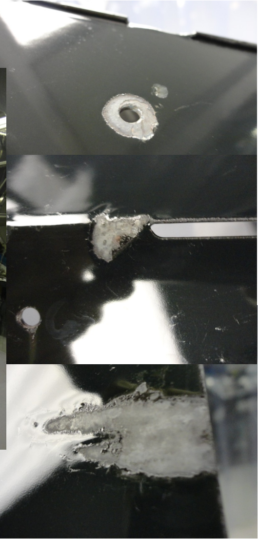
Pictures to the right: Spots where coating has already chipped off.
